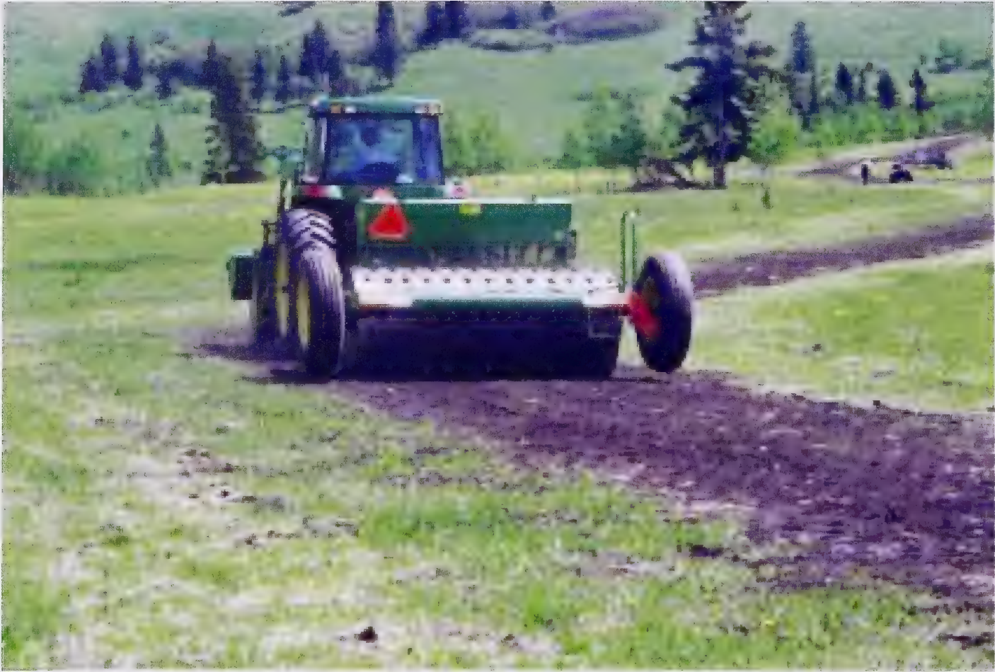
Photo 54 Kinsella Accuroller - seeds, packs and imprints the right of way.
